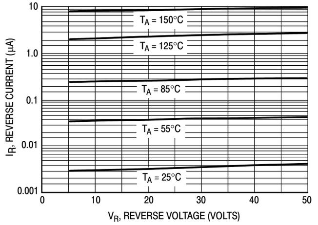
Figure 2. Leakage Current
