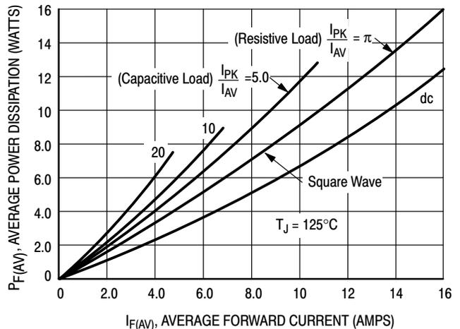
Figure 5. Power Dissipation
