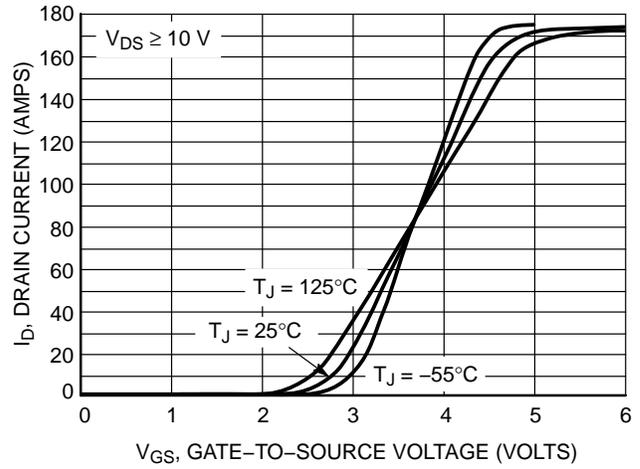
Figure 2. Transfer Characteristics
